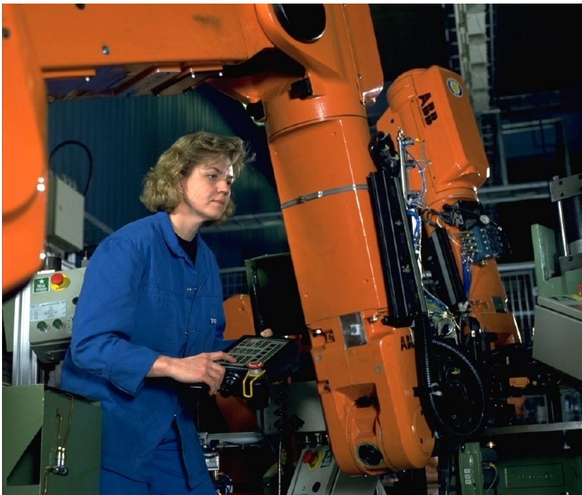
Figure 5 Robot operator/programmer at Volvo, using a hand-held terminal for on-line changes. (With permission from Volvo and ABB).
