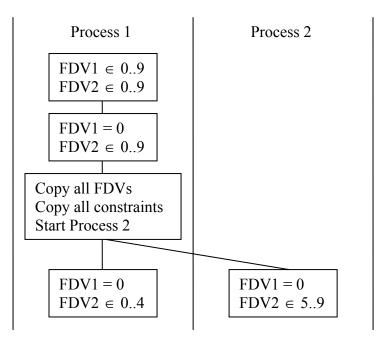
Figure 8: The parallelization procedure.
