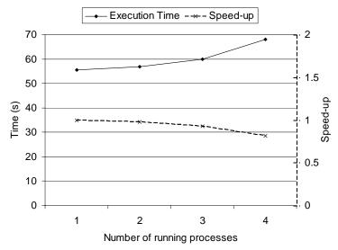
Figure 17: Execution time and speed-up when searching for one solution to Queens-500.
