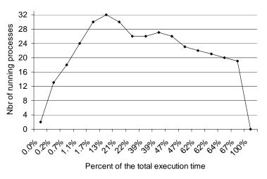
Figure 16: Load balancing for Golomb-11 when using 32 machines.
