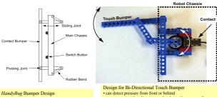
· rotational and sliding pivot points allow the bumper to react to pressure from any forward direction  can detect pressure from front or behind
