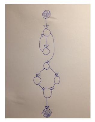
Figure 3.3: An Example of a control flow graph
